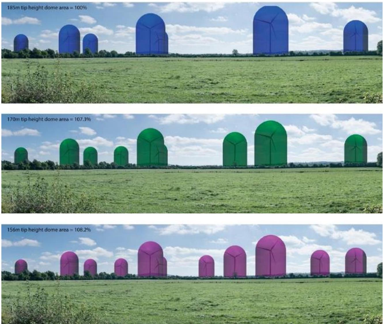
**Figure 2-2: Turbine Height versus Density Relationship (Same Power Output for each Example)**
